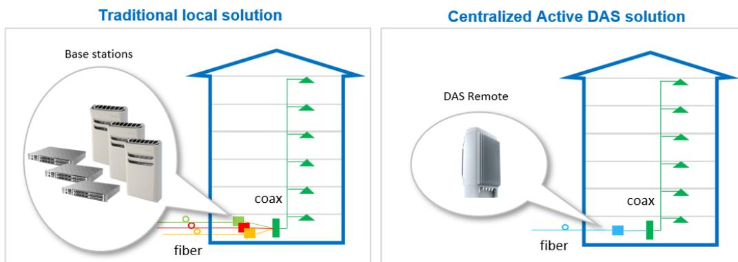
*Comparison of the local and centralized coverage solution*
